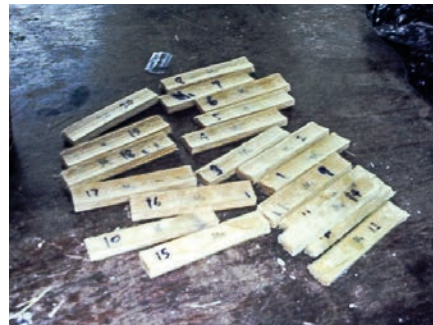
3.9: Bamboo samples for shrinkage determination
